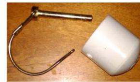
I use the 5 foot length of pipe and end caps to store and transport the antenna, a Comet SB14. To hold the end caps in place during transportation of the antenna I use a 1/4 -inch pin. Once
