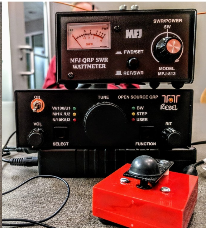
KB1TIC's complete QRP CW station
